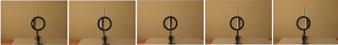
Figure 6. The part of the bar seen through the lens is seen infinitely far away (no left shift during the observers move from the left to the right).
