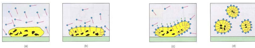
Figure 4. A submicro representation of emulsification.
